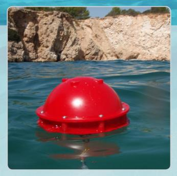
ODi are small and compact surface drifters to track sea currents based on Iridium, a global full ocean coverage bidirectional satellite communication network.
