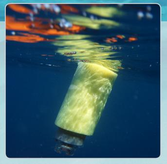
MD03 are small and compact surface drifters to track sea currents based on SMS GSM communication network.
